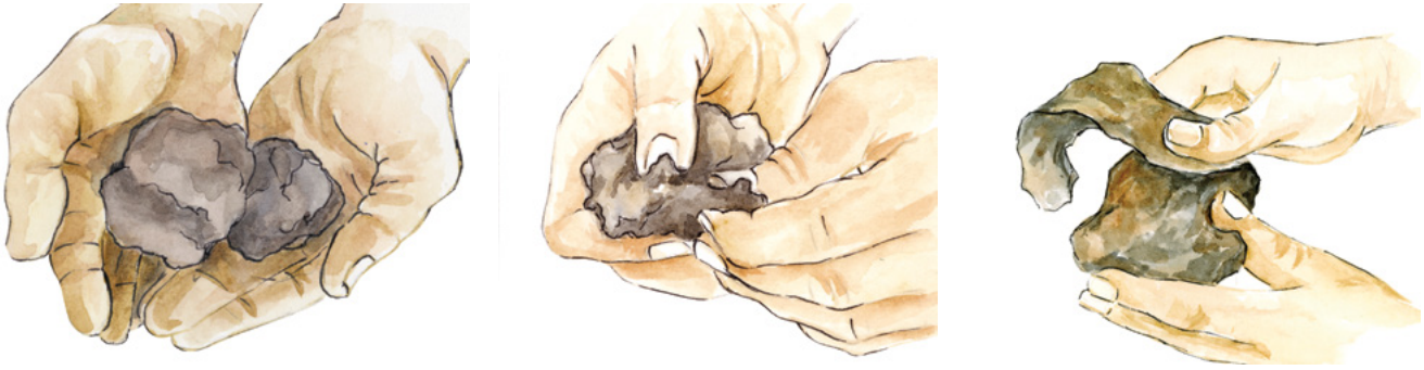
Figure 3-9: Texture by “feel” test
