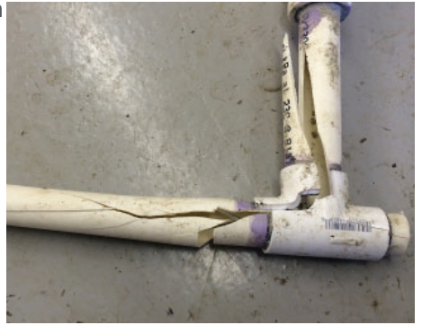
Figure 6-3: Broken PVC pipe from freeze damage.
