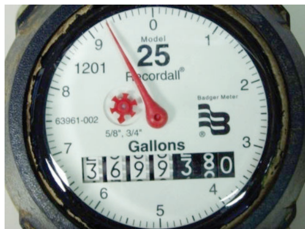
Figure 1-9: Straight-reading meters in gallons (upper) and cubic feet (lower)
