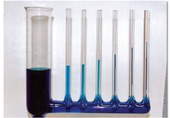
Figure 3-13: Capillary action (image courtesy of United States Department of Agriculture)
