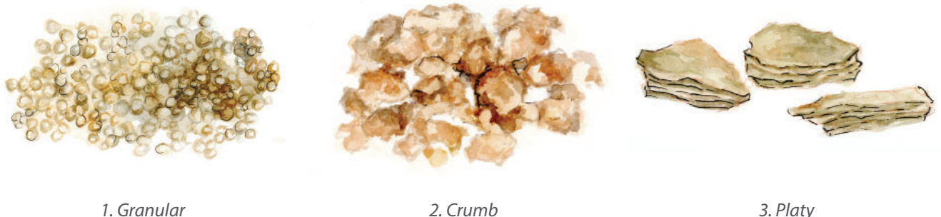
Figure 3-10: Soil structure from left to right (1) granular, (2) crumb, (3) platy
