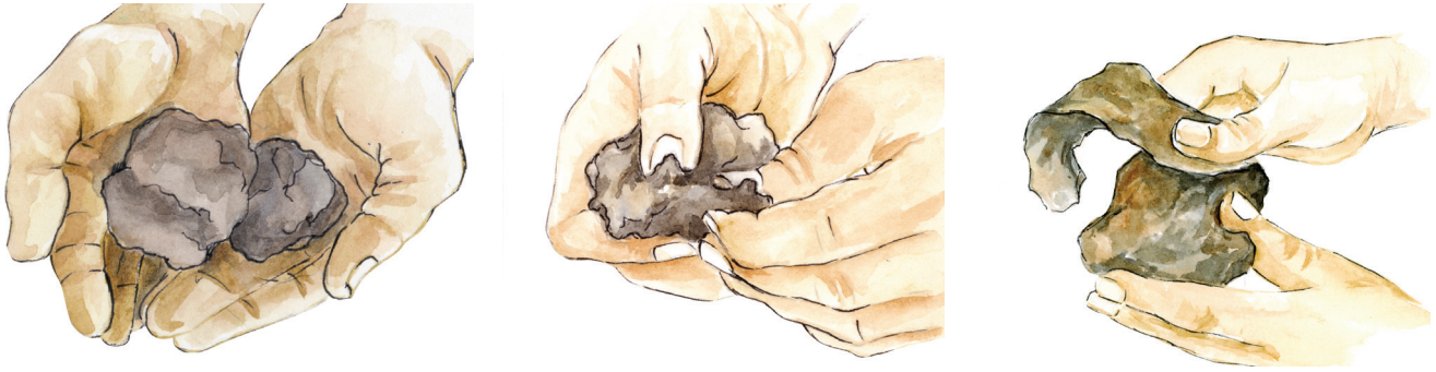
Figure 3-9: Texture by “feel” test
