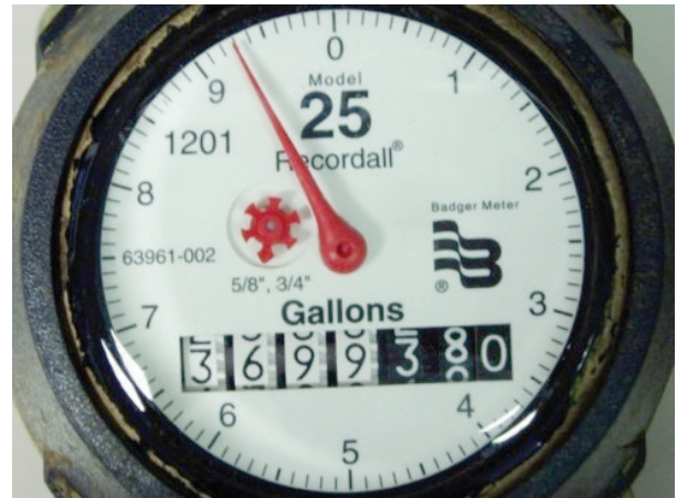
Figure 1-12: Straight-reading meters in gallons (upper) and cubic feet (lower)
