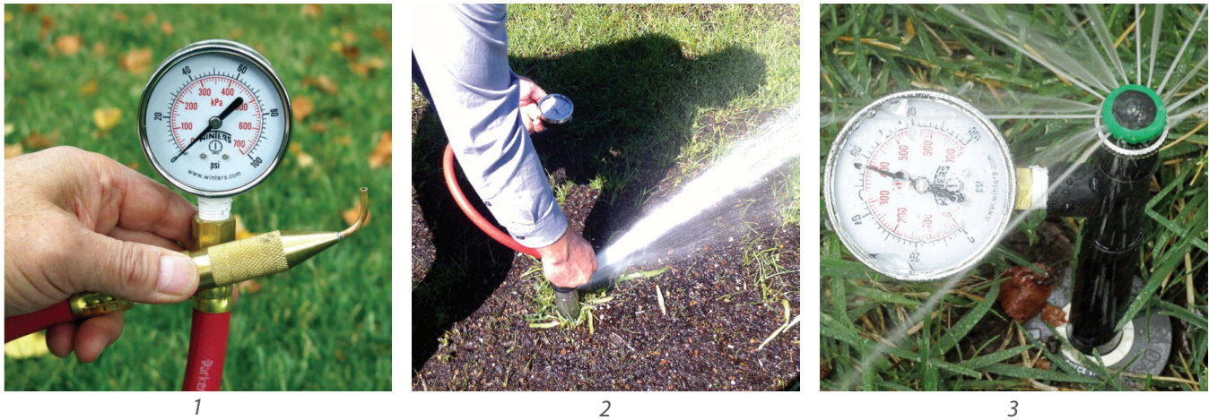
Figure 7-11: Left to right (1) pitot tube, (2) measuring pressure with a pitot tube, (3) gauge mounted to a tee
