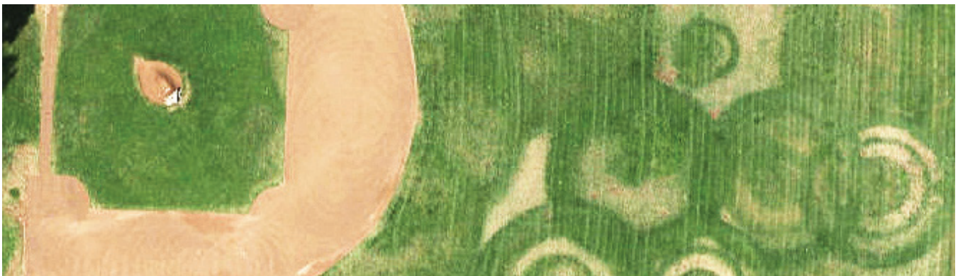
Figure 7-1: Irrigation circles on a sports field, a common indicator of poor DU
