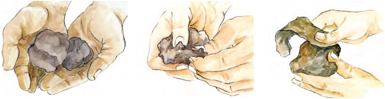
Figure 3-9: Texture by “feel” test
