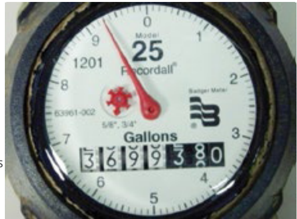
Figure 1-13: Straight-reading meters in gallons (upper) and cubic feet (lower)
